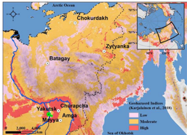
図1. Locations of candidate target areas in Eastern Siberia. The background map is a distribution of geohazard indices based on risk assessment of thermokarst subsidence (Hjort et al., 2018; Karjalainen et al., 2018).
