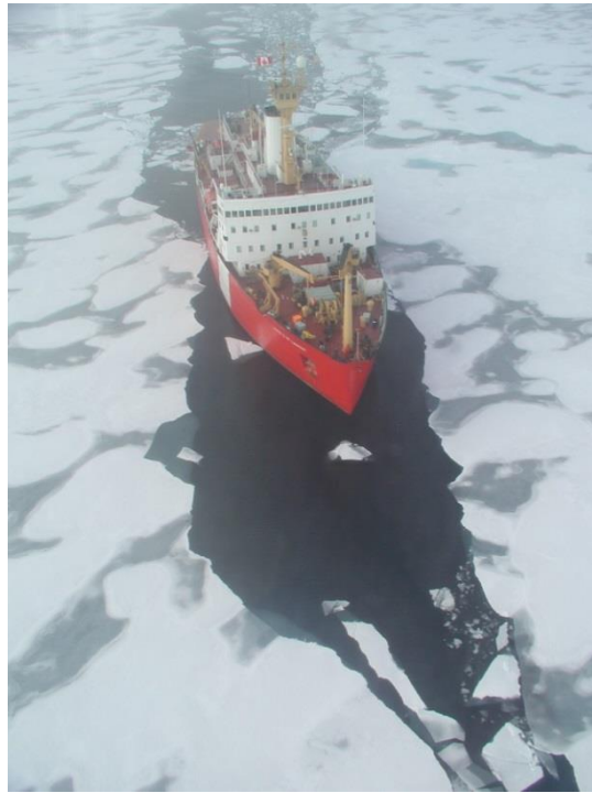
A Canadian research icebreaker advancing in the process of ramming icebreaking (Image courtesy of Koji Shimada)
